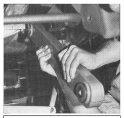
The big lower trailing arms are really impressive, especially against the stock arms. The arms are heli-arc welded for strength and the powder coating will last a very long time. Grease zerk fittings are also included on the Hotchkis trailing arms, which may also be purchased separately.
