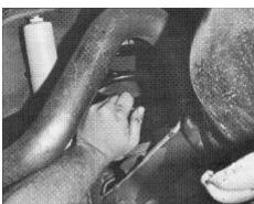
The new Bilstein shocks were installed to their top mount first. This way we can still install the new rear springs, then the lower shock mounts, without getting up.
