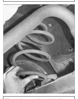
When you've removed or unbolted the lower attachment of the shocks you can jack up the body and remove the rear springs.
