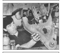
Two bolts through the rubber bushings hold the lower A-arm in place.
