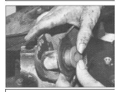
The new Energy urethane bushing slides smoothly in place of the stock rubber piece.
