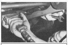
The factory sway bar mounts in the exact same position as bolt accommodations on the Hotchkis arms.
