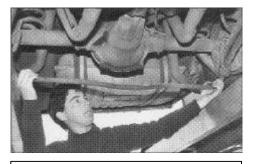
The rear suspension revamp begins by removing the sway bar. Two bolts hold it to each lower trailing arm.
