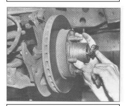
Next, remove the brake rotor and set it aside. Be sure not to mix up the right and left bearings, and keep dirt and other debris out by covering with a clean rag. You should also repack with high-temp wheel bearing grease when you reinstall.
