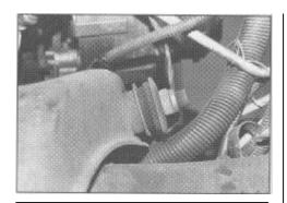
The 10-year-old stock rubber bushings on our Buick were very worn. The inside of this bushing really deteriorated due to heat from the turbo pipes that pass close by. The bushing had gotten so bad the shaft was loose and making lots of clunking noise.
