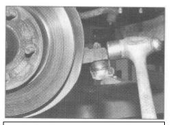
Loosen the nut to remove the outer tie rod end from the spindle. If it won't release, give it a light tap with a hammer as seen here.
