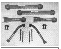
The Hotchkis high-performance rear axle control system (part # 1802) consists of upper and lower rear trailing arms, tubular trailing arm braces, urethane bushings and hardware. This system with its boxed steel tube trailing arms allows the rear suspension to resist flexing associated with wheel hop on hard launches. The trailing arm braces tie it all together and improve cornering as well. The kit is available in red or black powdercoat.
