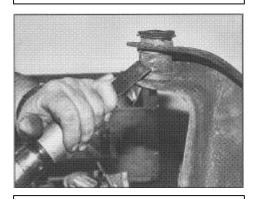
Once again, an air chisel made quick work of the stock bushing. Remember to pry the old bushings out in the proper direction according to the lip of the bushing case, usually on the outside.
