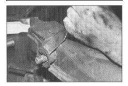
An air chisel makes bushing removal easy.
