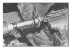
Install the washer over the end of the bushing and bolt the nut onto the shaft using an impact or heavy socket wrench.
