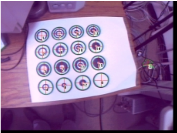
Figure 2. Example of ring detection and identification for 4-bit markers.
